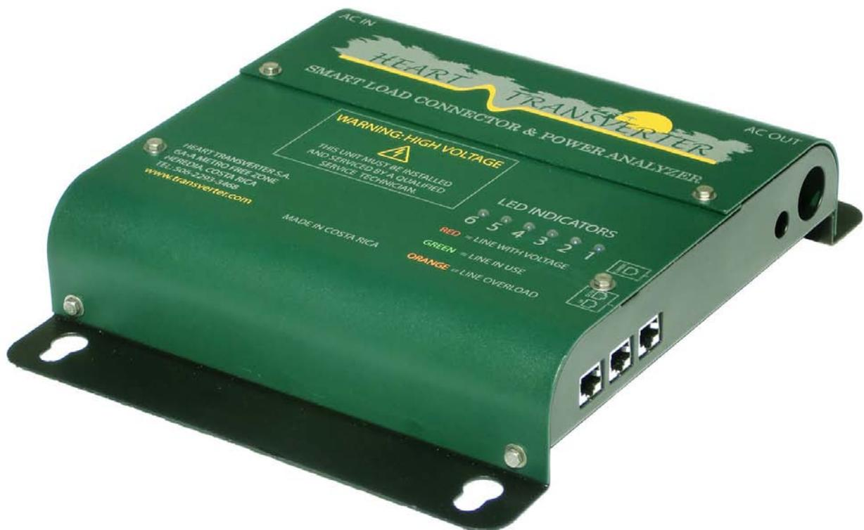
**The Product.** The Transverter T13X has connections for 4 line voltage sense lines and inputs and outputs for six 30 amp relays. It has a Cat5 cable connection that goes to a small connector module which connects to up to four snap on current sensors for the 100 amp main grid inputs. It also has a
