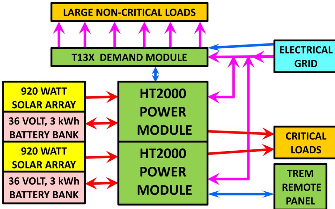
A Transverter System as described above, allows you to integrate solar panels directly into the UPS system so that, during daylight hours, the solar is providing energy directly to the resident’s UPS critical loads and recharging batteries.
